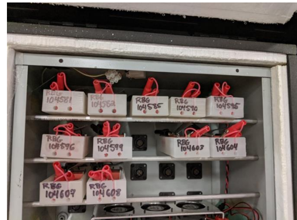
Pouch cells in a temperature box (40°C)
